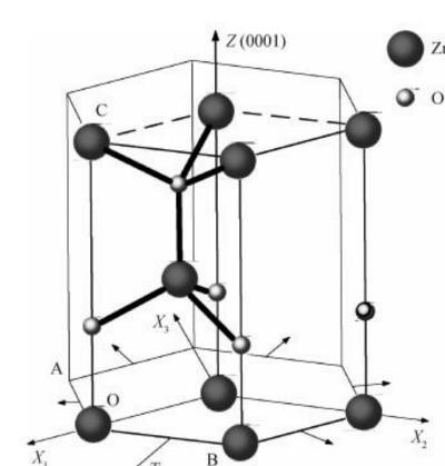
ZnO shown here, has a no centrosymmetric wurtzite structure, and has a spontaneous electric polarization, but does not switch in response to an applied electric field (not ferroelectric)
